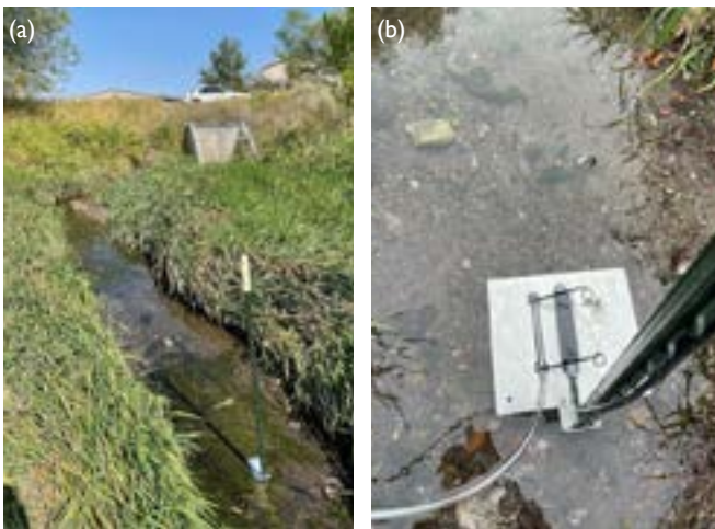
Figure 5. Location along channel at KAL_AC6 to test automatic sampler. (a) T-post and bracket at exact sampling spot. (b) Sensor plate connected to T-post bracket with area-velocity sensor and sampling tube and strainer mounted. Pictures taken August 30, 2021, and September 28, 2021, respectively.
