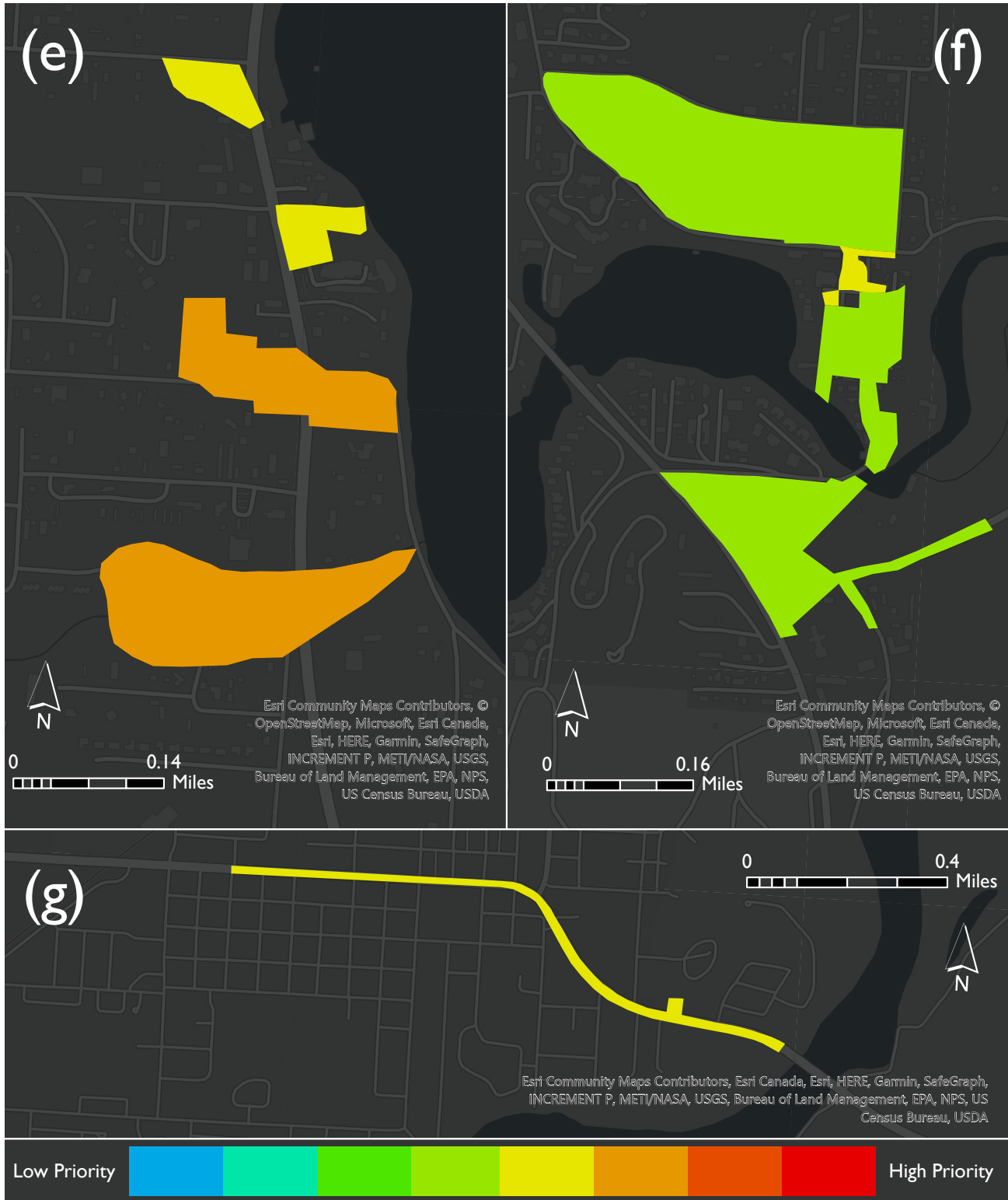
Figure 2. Results of the 2021 outfall prioritization model in (a) Kalispell and Evergreen, (b) Whitefish, (c) Polson, (d) Ronan, (e) Lakeside, (f) Bigfork, and (g) Columbia Falls. High priority sub-basins (cumulative score of 6 or 7) are labeled. Projected Coordinate System: NAD 1983 (2011) StatePlane Montana FIPS 2500 (Meters).
